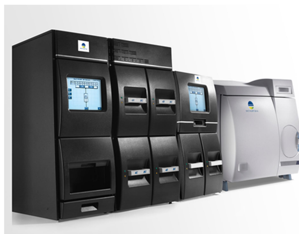
Figure 12 : Automate BacT/ALERT® 3D
