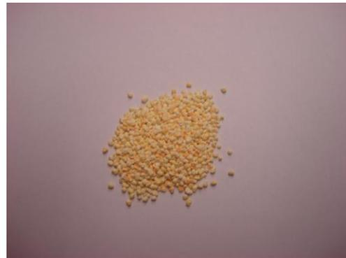
Figure 34: Photo des grains chargés  $710 < d < 1000 \mu\text{m}$
