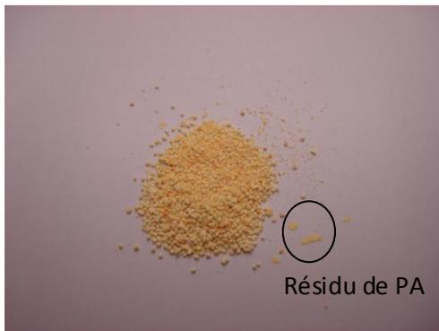
Figure 33: Photo des grains chargés  $500 < d < 710 \mu\text{m}$
