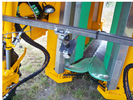
FIGURE 4.9 – Le radar Doppler installé.
