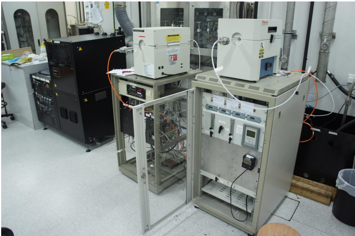
Fig. 36. CVD systems in NEL2, School of EEE, NTU
