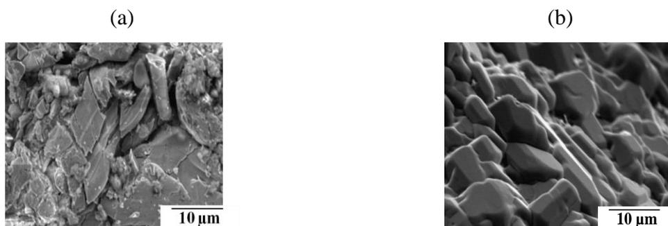
**Figure 5.** photos MEB des compositions (a)  ${}_{0,18}^{25}\text{G}_{0,5}^{\text{M125}}$  et (b)  ${}_{0,18}^{25}\text{G}_{0,5}^{\text{T125}}$
