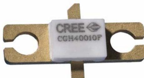
**Figure 145:** Transistor CREE GaN CGH40010F
