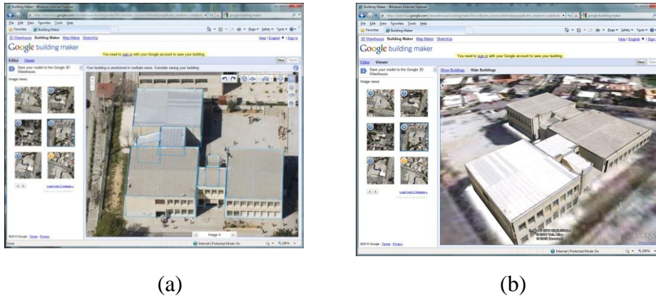
Figure 17: (a) Constructing a model with “Google Building Maker” (b) 3D reconstructed model of building (“Building Maker” process)
