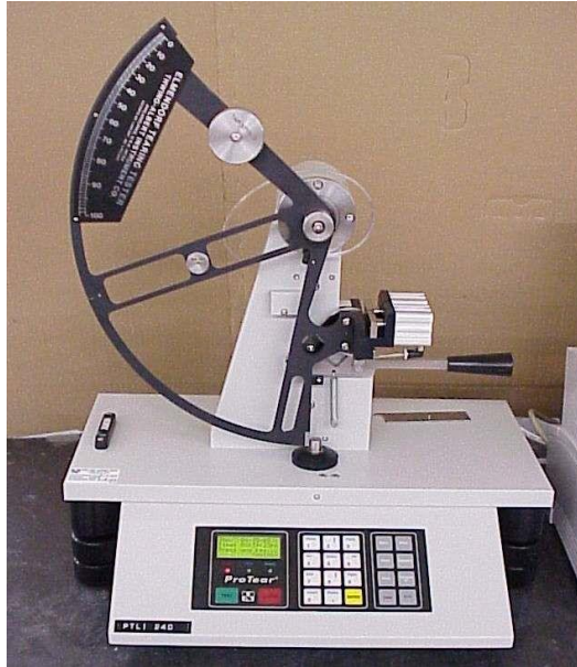
Figure 1.5.2.3.a : Elmendorf Tearing Tester Thwing-Albert.
