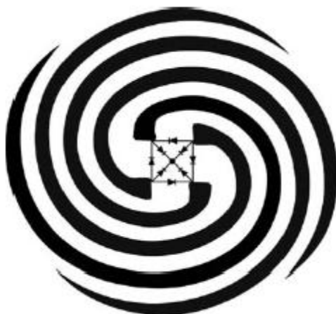
Figure. I.11. 4-arm spiralphase circularly polarized reflectarray with switching diodes in the center
