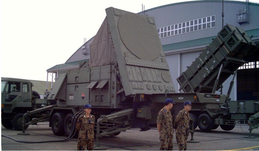
Figure. I.8. A closer look to the AN/MPQ-53 PESA radar installed in the patriot systems
