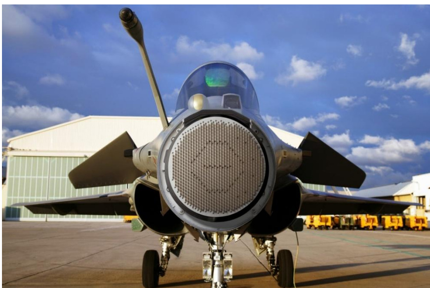
Figure. I.9. RBE2 radar installed inside the RAFALE combat aircraft
