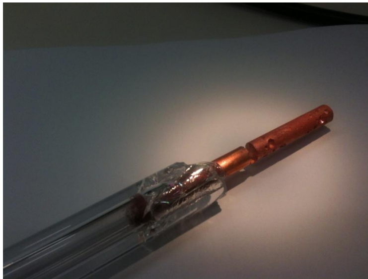
Figure 3.22: Photograph of the first realization of a copper preform using the vitrification unit
