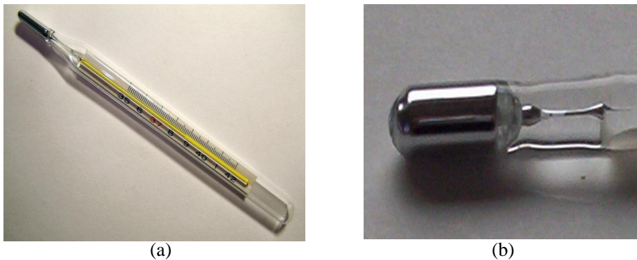
Figure 3.11: (a) Clinical thermometer (b) Break in narrow region
