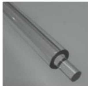
Figure 1.7: Representation of the rod in tube method
