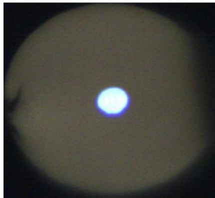
Figure 1.15: Doped \text{GeO}_2 silica core (88% \text{SiO}_2 and 12% \text{GeO}_2 ) silica cladding fiber [61]
