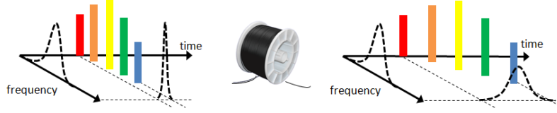
Figure 2.10: Pulse spreading due to chromatic dispersion .
