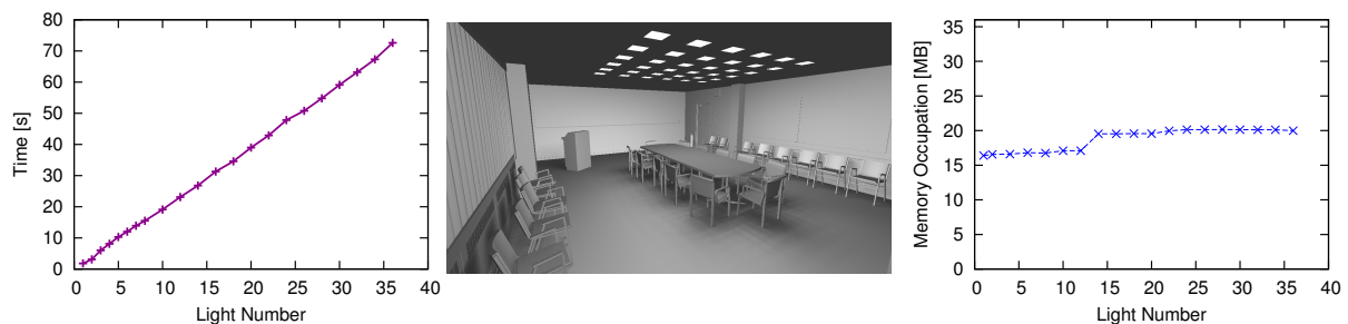
Figure 2.21: Increasing the number of lights. Left: The time consumption. Right: The maximum memory load reached during the computations. Center: A picture from our tests with 36 area light sources.
