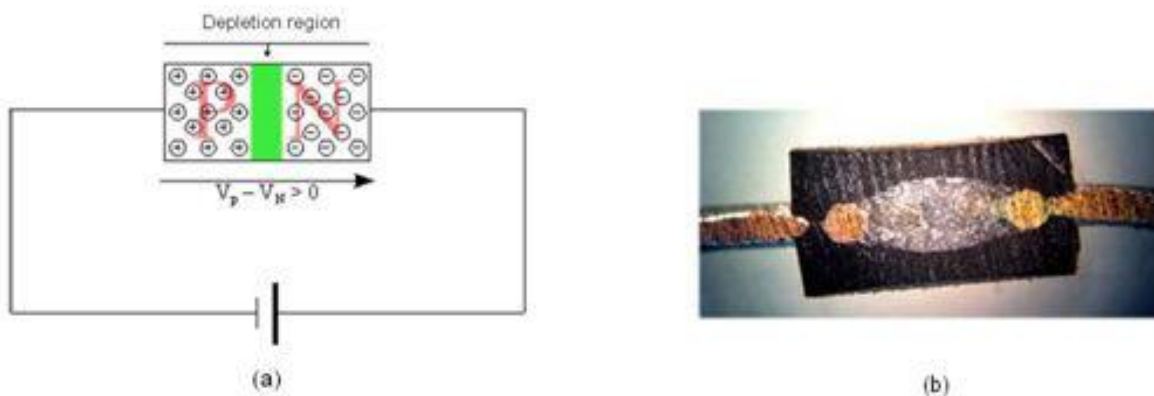
Figure 3-6: (a) schematic design and (b) section photo of the PCSS used for the generator.
