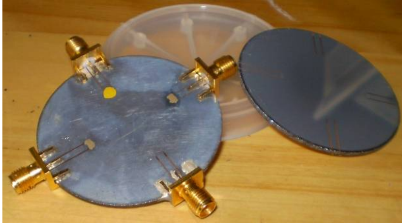
Figure 2.13: Photograph of the fabricated sample with the SMA connectors mounted and materials deposited.
