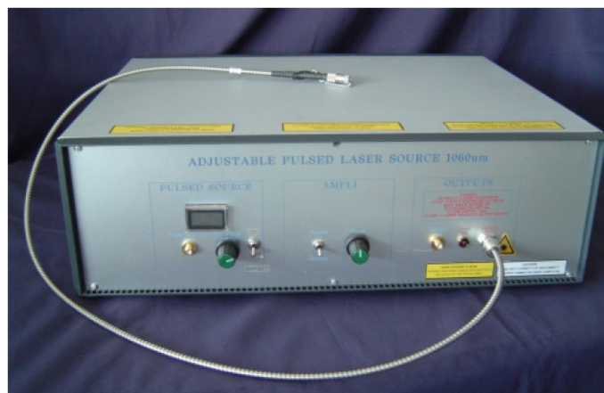
Figure 5.2: Picture of the complete adjustable laser source.
