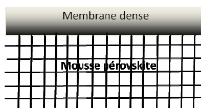
Figure 17 Architecture membrane dense sur support mousse pérovskite
