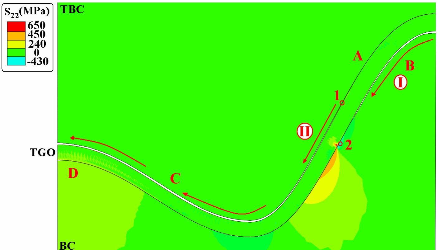
Figure 4-8. Crack development scenario in the case of 3 \mu\text{m} TGO thickness in the TBC/TGO and TGO/BC interfaces for two amplitudes non-uniform after cooling.
