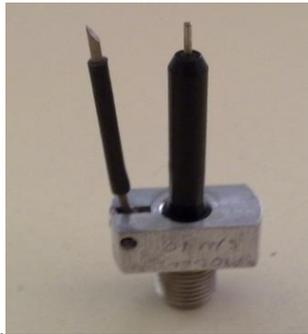
Figure II.20: Sonde haute tension (2440, Barth Electronic Technology, USA)
