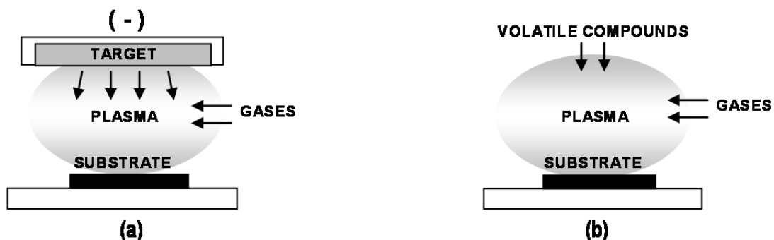
Figure 1.7: General sketches of the PAPVD (a) and PECVD (b) processes.
