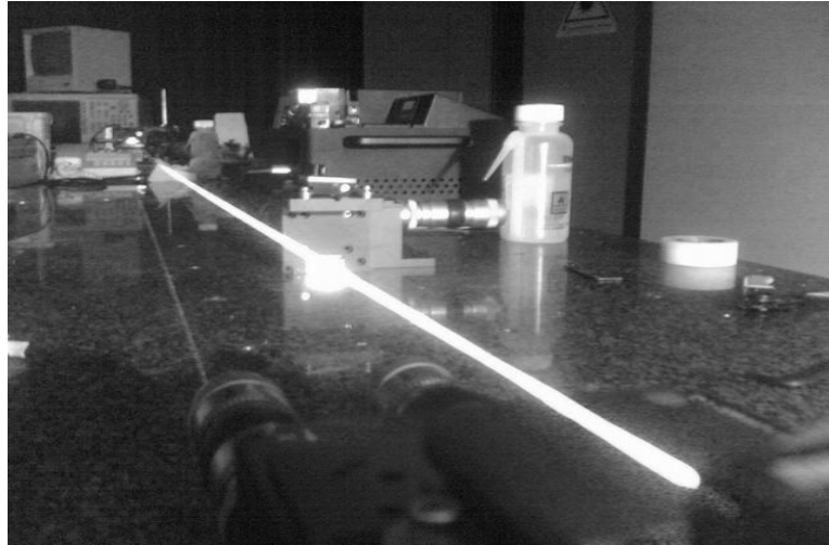
Fig. 29: Working fiber laser based on 2 m length BF in experimental scheme shown on Fig. 28.
