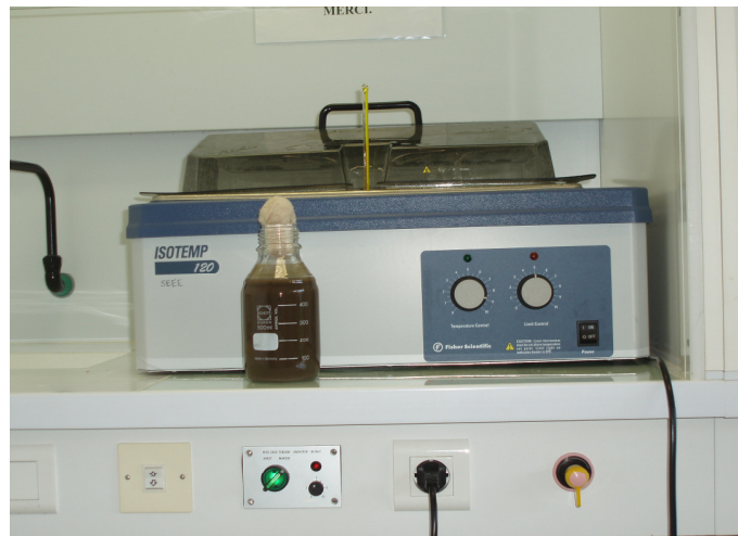
Figure 2-3: Photo of Bain- Marie reactor for thermal treatment.
