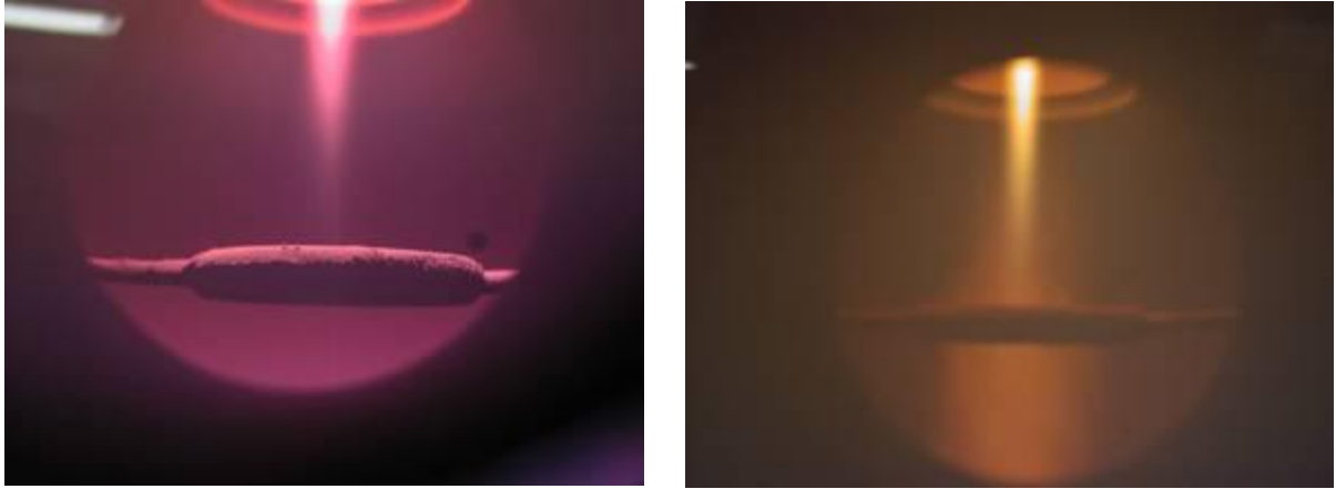
Figure 3-12: left: plasma without particles. Right: plasma with Si particles. In both cases the plasma conditions were the same. The pictures show the quench ring and the transition from torch to synthesis chamber at the top. In both cases the plasma flows from top to bottom. Distance top plasma to quench ring amounts 121 mm.
