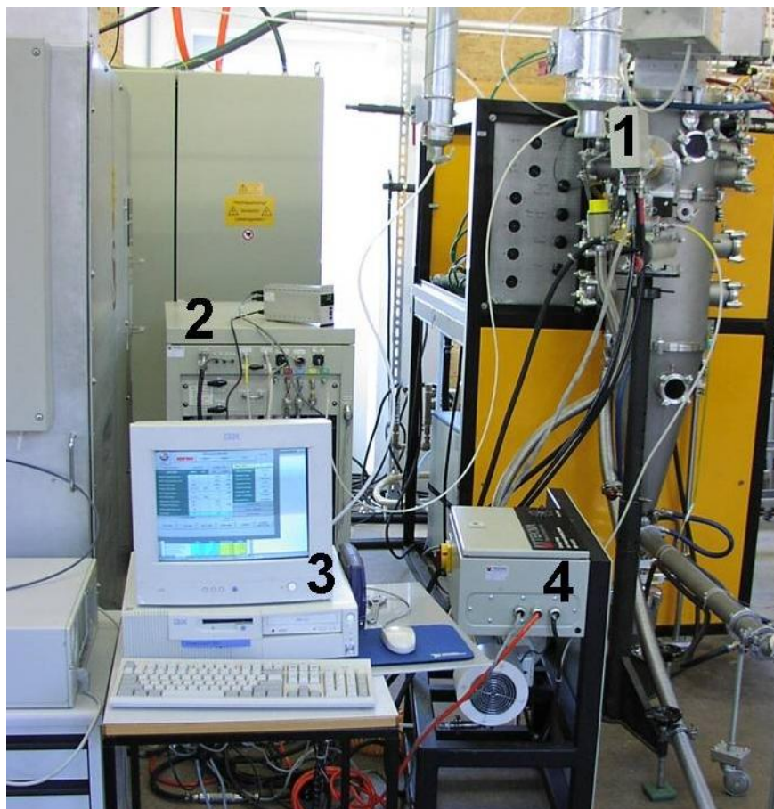
Figure 3-17: Picture of enthalpy probe set-up: 1) bulk head, 2) console, 3) computer with special software, 4) pump.
