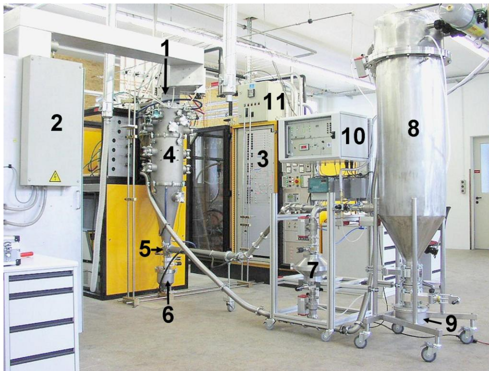
Figure 3-1: overview of the ICP equipment. 1) torch, 2) RF power supply, 3) gas control unit, 4) synthesis chamber, 5) T-junction, 6) micron powder collector, 7) nano- particle sampling filter, 8) production filter, 9) production collector, 10) filter control unit, 11) water cooling control unit.
