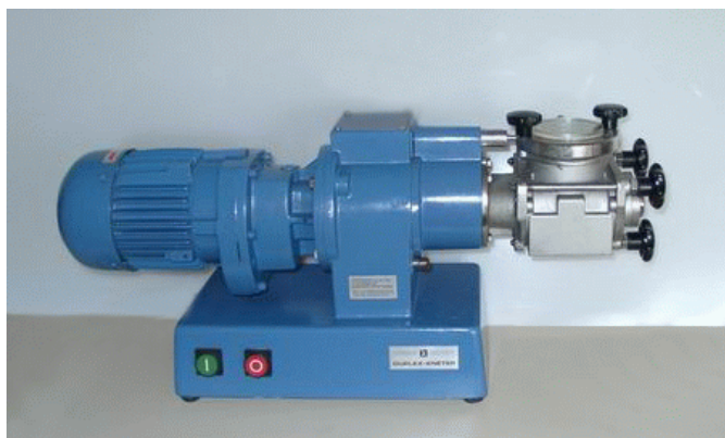
Figure 19. Labo-Reactor System (on the left image) and mixer with Z-blades (on the right image).
