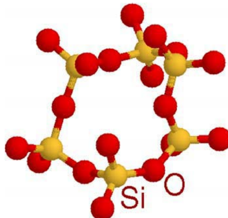
Figure 1.1 : structure de la silice [Hu-1]
